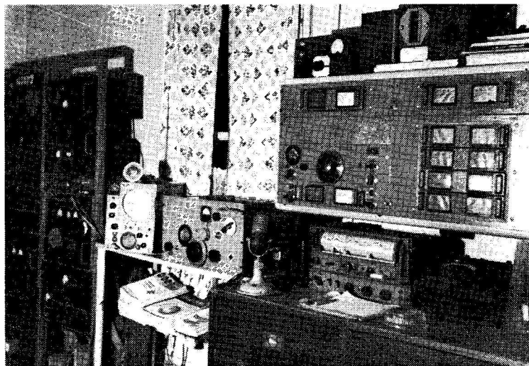
Licensed in November, 1955, G3KPW (Askern, Yorks.) started up on 80 metres, since when the station has been greatly expanded and much gear built. The main transmitter now runs 150w. to an 813, over 80-10 metres, modulated by a pair of TZ40's, and the receiver is a rebuilt and miniaturised HRO, incorporating a product detector and noise limiter, with a lattice filter under construction. A prototype SSB rig using the phasing mode is in hand. For aeriols, G3KPW has a 132ft. wire, a 20-metre dipole, and a 3-element Minibeam, with a Cubical Quad for 10-15 metres projected — if he can keep it airborne, two having been lost so far! As the photograph shows, the station is also fully equipped with test gear and ancillaries.
